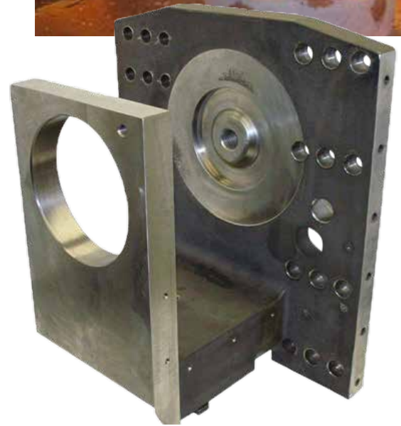
Finished Machined Forkroller 20"x20" 290 lb
